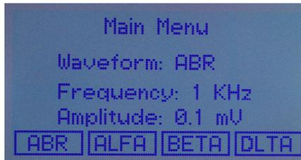
The desired amplitude can be selected by pressing the “AMP” key and using the F1, F2, F3, F4 keys. Use the <, > keys for more amplitudes.
