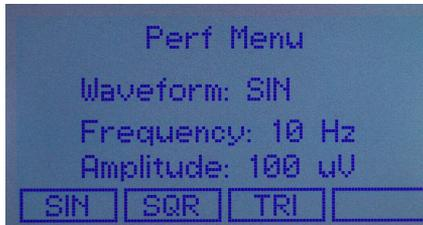
Select any of the desired waveform using the F1, F2, F3 keys.
