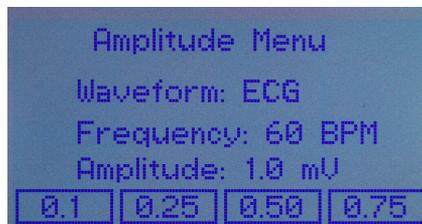
To change the ‘Amplitude’, press “AMP” key and any of the F1, F2, F3, F4 Keys for the desired amplitude.
